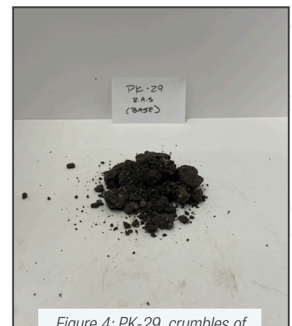
Figure 4: PK-29, crumbles of unbonded base
